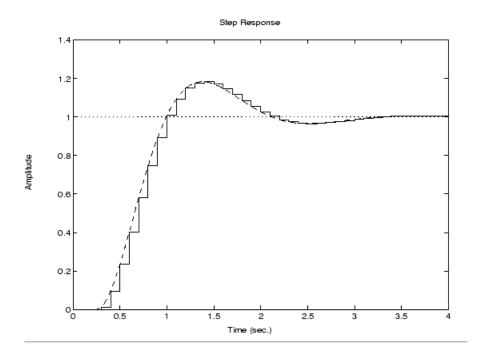
Discretize a state-space model with time delay, using a Thiran filter to model fractional delays:
