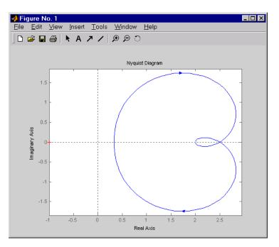
The nyquist function has support for M-circles, which are the contours of the constant closed-loop magnitude. M-circles are defined as the locus of complex numbers where
