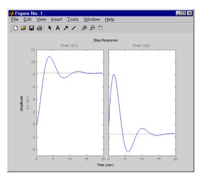
The left plot shows the step response of the first input channel, and the right plot shows the step response of the second input channel.
