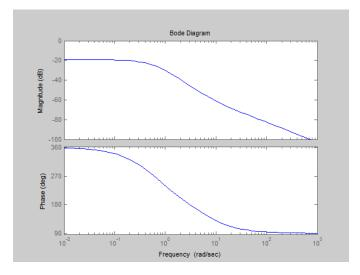
bode (sys1,..., sysN) plots the frequency response of multiple dynamic systems in a single figure. All systems must have the same number of inputs and outputs.
