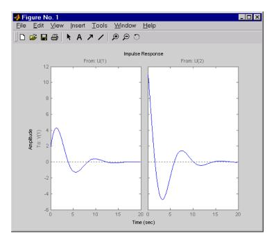
The left plot shows the impulse response of the first input channel, and the right plot shows the impulse response of the second input channel.
