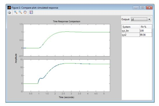
sys2 provides a 99.93% fit for the first output and a 98% fit for the second output while using 4 less states than sys\_lin.
