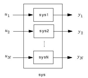
For systems with transfer functions  $H_1(s), \ldots, H_N(s)$ , the resulting system sys has the block-diagonal transfer function
