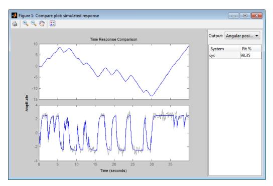
$\mathsf{sys}$  provides a 98.35% fit for the angular position and an 84.42% fit for the angular velocity.
