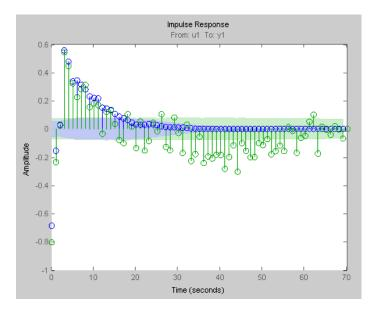
The uncertainty in the computed response is reduced at larger lags for the model using regularization. Regularization decreases variance at the price of some bias. The tuning of the regularization is such that the bias is dominated by the variance error though.
