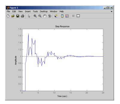
**Note** The system step response displayed is chaotic. The step response of systems with internal delays may exhibit odd behavior, such as recurring jumps. Such behavior is a feature of the system and not software anomalies.
