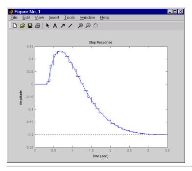
Discretize the delayed transfer function
